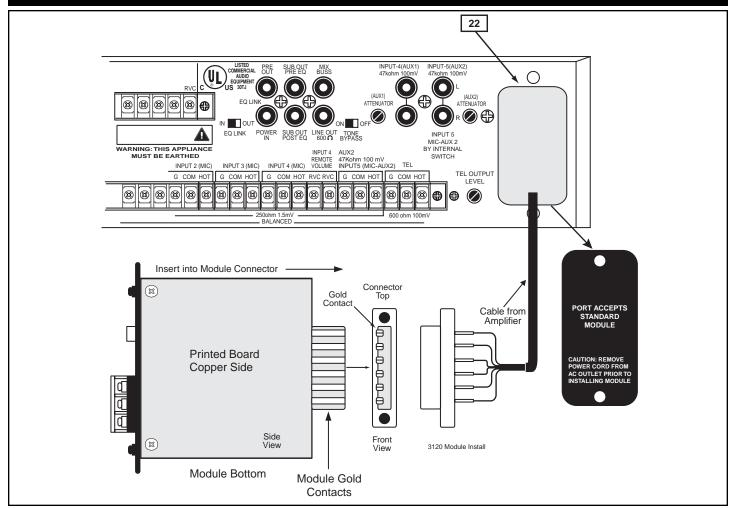
Fig. 22 - Rear Panel Module Installation Diagram
